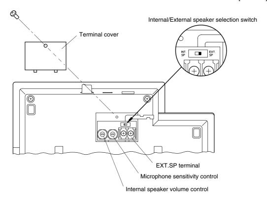
Step 2. Connect the speaker cable to EXT.SP terminal.
